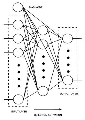
Fig. 1. General structure of a feed-forward network with one hidden layer.
