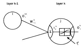
Fig. 2. The structure of a node in the hidden and the output layer.
